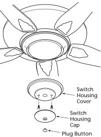
Figure 7a - Removing Plug Button and Switch Housing Cover
